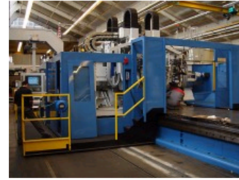
RECONSTRUCTION AND TRANSFORMATION OF A MILLING. MANUFACTURE OF TWO MILLING HEADS TO ADD ON THE MILLING.
